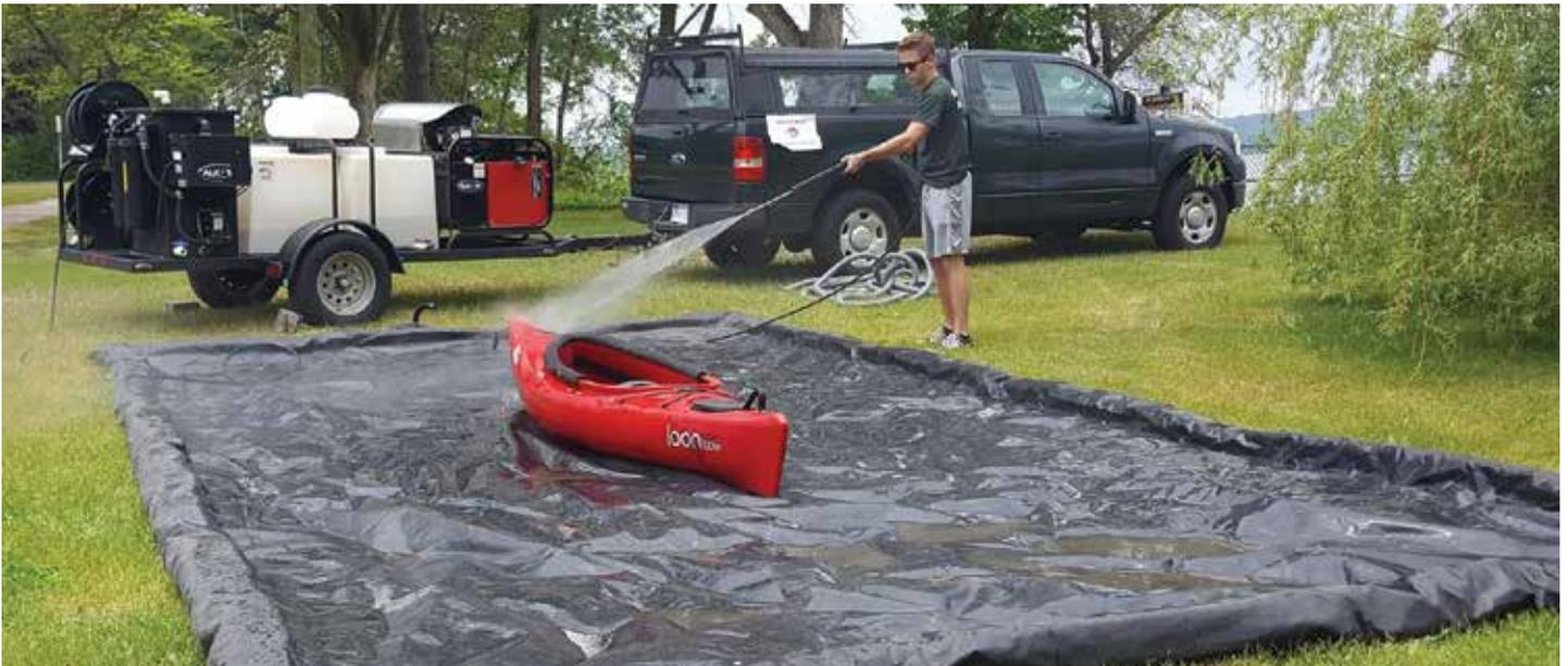
THE MSU MOBILE BOAT WASH IS A HOT WATER, HIGH PRESSURE WASHING UNIT ON A TRAILER.
