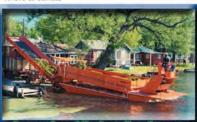
Transport Barge Offloading to Shore Conveyor
